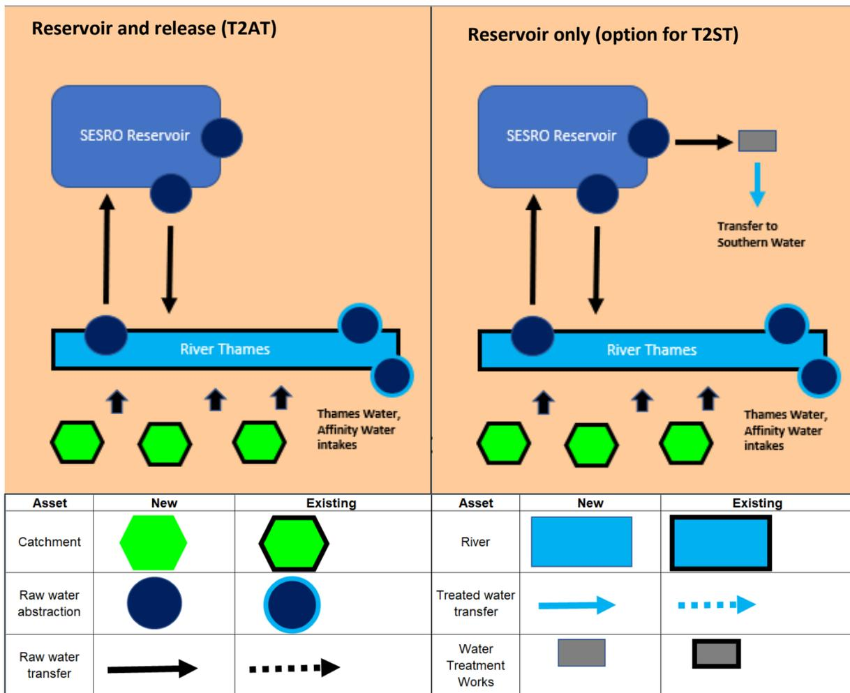
Figure 2.1 WQRA spreadsheet schematics for Thames to Affinity Transfer (T2AT) and Thames to Southern Transfer (T2ST)
