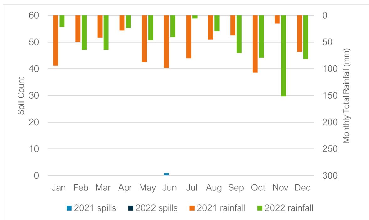
A trend in spill performance at Basingstoke STW cannot be established based on the above data, as only one spill was recorded at the site in 2021, and no spills were recorded in 2022. Please refer to the Groundwater Impacted System Management Plan for 2021/22, included in this PDF document, for discussion regarding trends evident in the EDM data for 2020, indicative of the role of groundwater infiltration on spills in the catchment.
