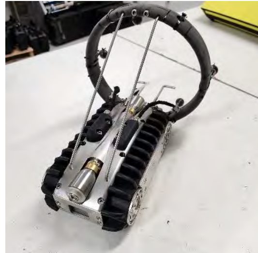
Figure 2. Completed build with accelerometers mounted on the halo to the rear
