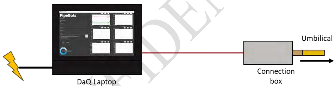
Figure 4 DaQ arrangement for sensor data collection.
