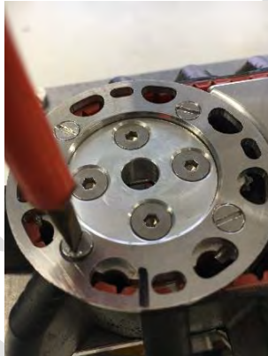
Figure 12 Remove a) retaining plate screws & b) retaining plate.
