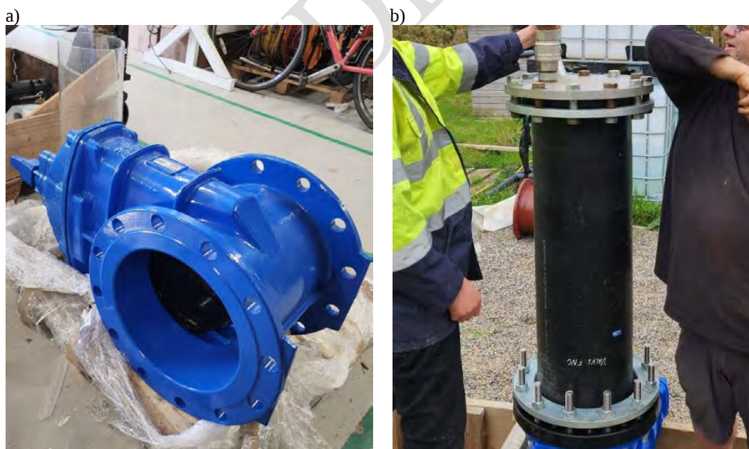
Figure 4 Live access equipment for pressurised tests showing a) the DN300 Donkin gate valve and b) the launch tube assembly connected to the Donkin valve on site.
