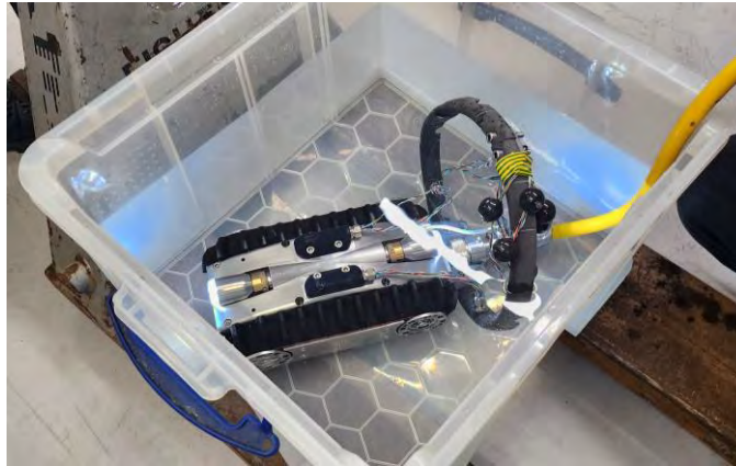
Figure 5 Crawler functionality and internal pressure testing when submerged in water.
