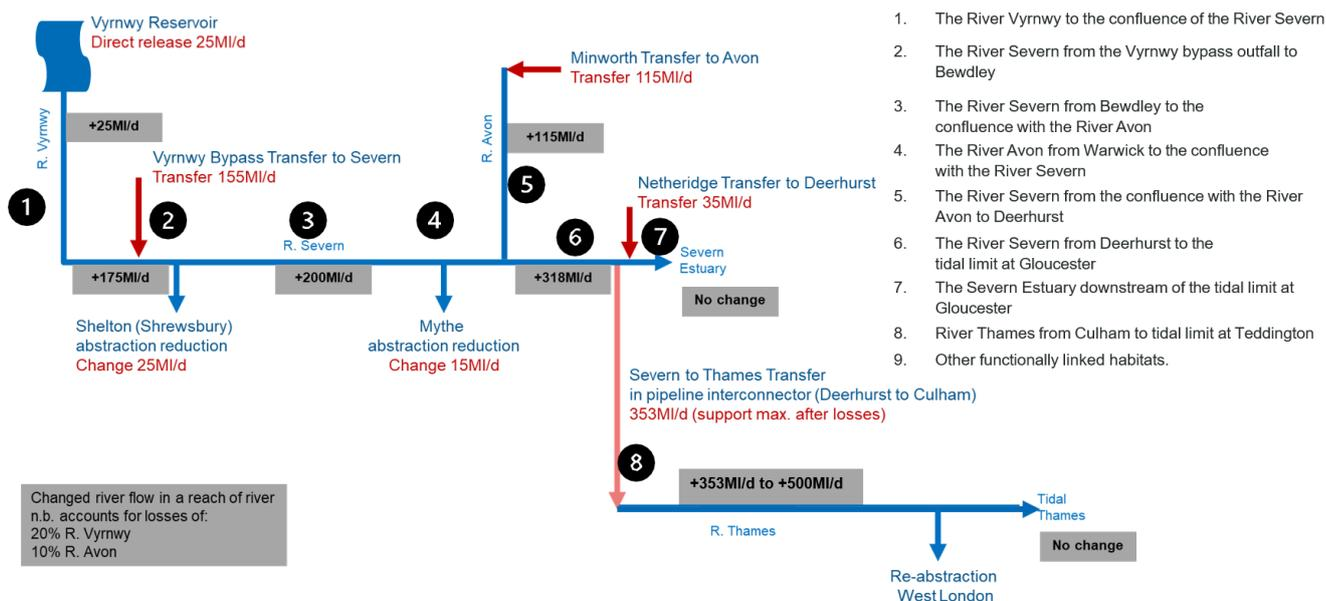
**Figure 1.3 Schematic representing flow changes (accounting for losses) of STT Solution**
