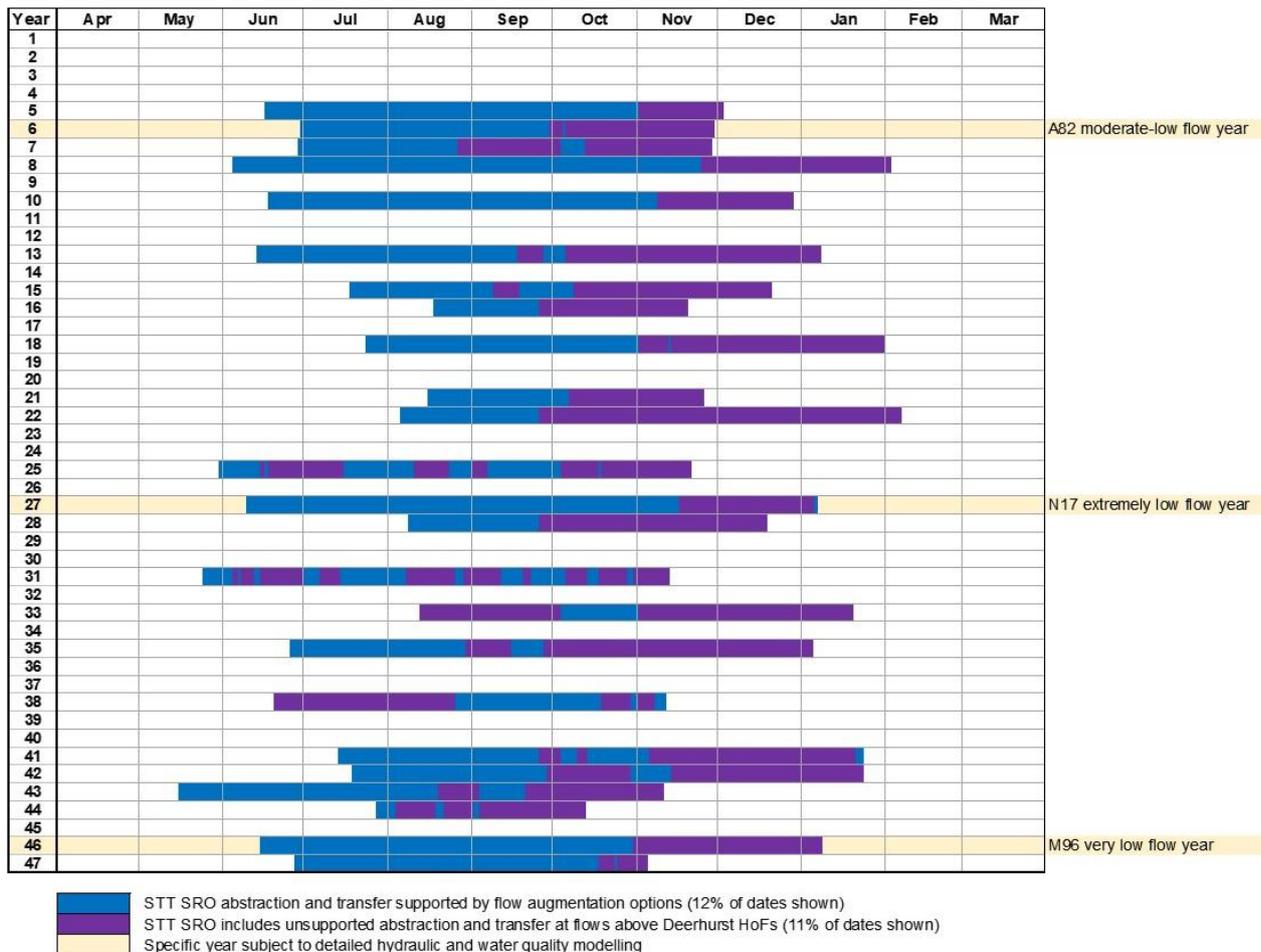
**Figure 1.4 Representation of dates full STT solution would be on (for water resources purposes) as used in environmental assessment**
