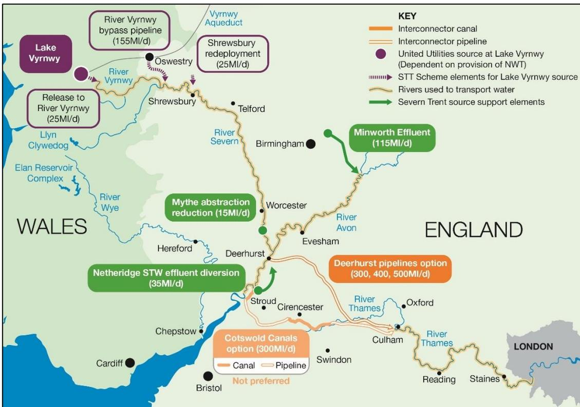
The Interconnector will transfer treated river water (unsupported flow) from the River Severn to the River Thames when there is a need. When the flow in the River Severn is insufficient or is
