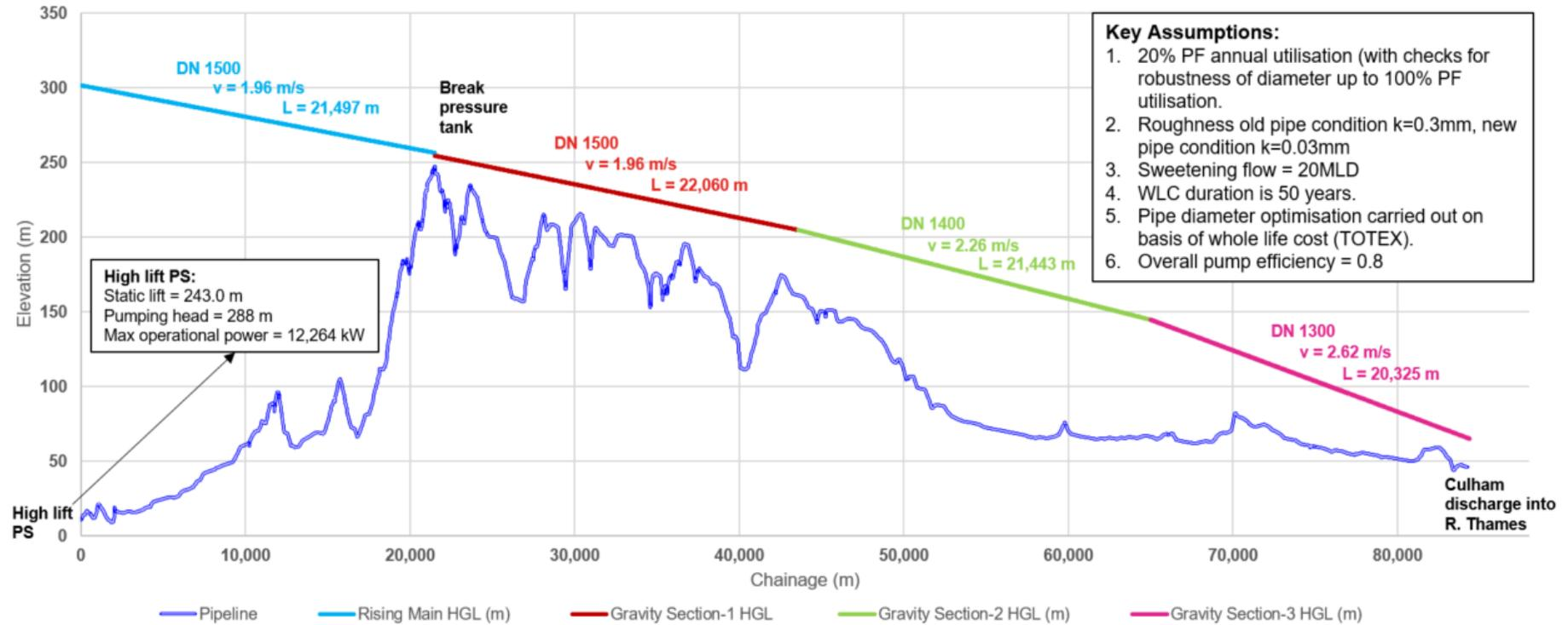
Figure 2.2: Transfer pipeline design details 400MI/d capacity option
