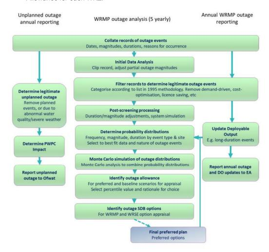
Figure J-1: Approach to Outage Allowance Calculation - Taken from WRSE Outage Method Statement
