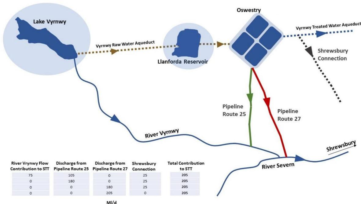
The Bypass pipeline is a gravity main pipeline and is contained within the licence area of Severn Trent Water. This will require limited operation and maintenance apart from an annual walk over inspection. The gravity main carries the treated water approximately 10.3 or 16.5 km from Oswestry to the river Vyrnwy or Severn discharge outfall (Figure 3-1). It is assumed to be a thin wall steel pipe. However, further assessment
