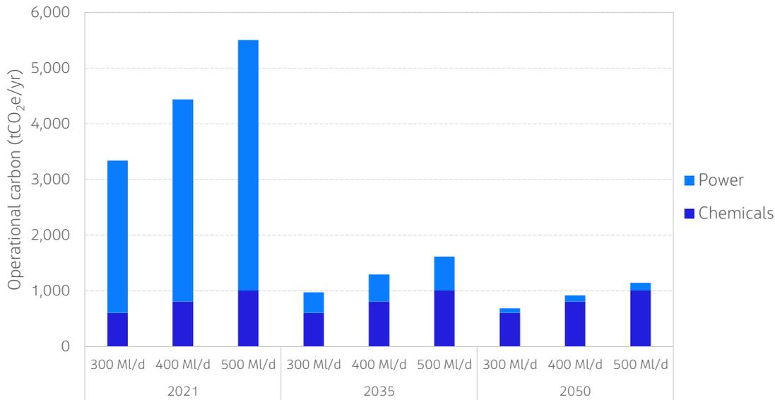
Power consumption is a significant emissions hotspot during the early operation of the STT. Over time the significance of power related emissions as the grid decarbonisation projects take effect. Figure 4-6 shows the projections of the emissions associated with the three different design options of the interconnector between now and 2050.
