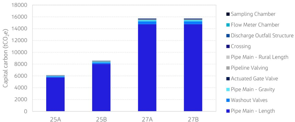
The next largest hotspot for the Vyrnwy Bypass Pipeline sub-options, is the capital emissions associated with the valves, including washout valves, actuated gate valves, and pipeline valving. These emissions total 3-4% of the capital carbon emissions. There are 4 other categories of capital carbon emissions, with a combined ~1% of the total capital emissions across the four different designs.
