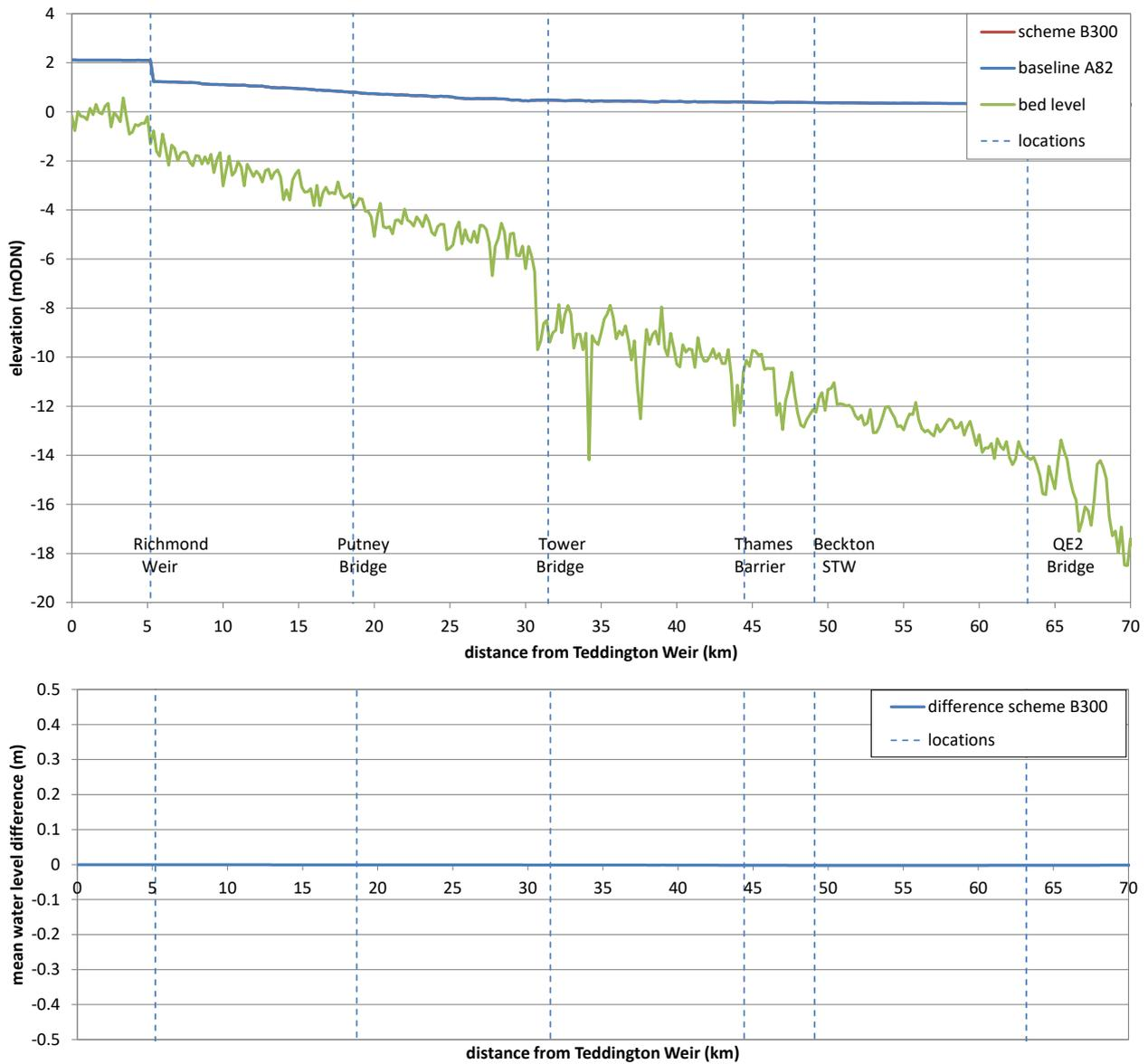
Figure 3-5 Mean water level along thalweg during scheme operation (6 August- 12 November), M96, baseline and B300 scheme, Teddington to QE2 bridge
