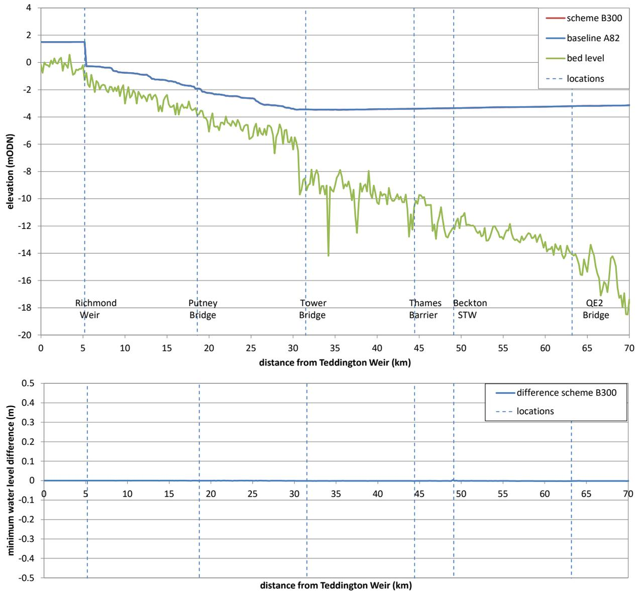
Figure 3-3 Minimum water level along thalweg during scheme operation (6 August- 12 November), M96, baseline and B300 scheme, Teddington to QE2 bridge
