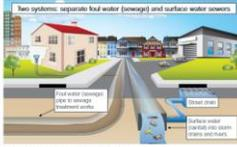
Two systems: separate foul water (sewage) and surface water sewers
