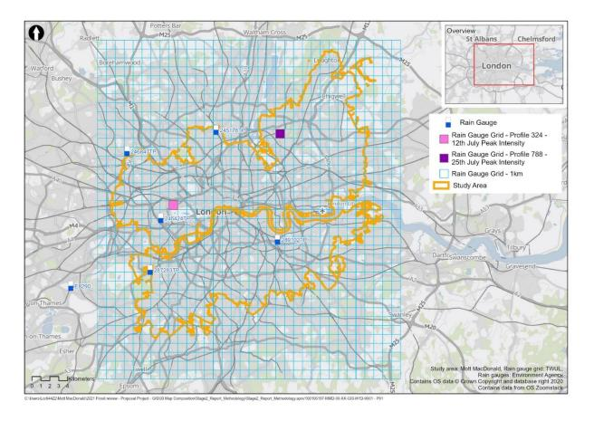
The data shows that the 12 July 2021 rainfall was much more significant in terms of total depth and intensity of the rain but affected a smaller area than the 25 July rainfall. On 12 July, the most severe rainfall was in Bayswater; on 25 July it was in Walthamstow. Both events were greater than the design standard for drainage systems. This refers to the likelihood of a similar flood event occurring in a given year.
