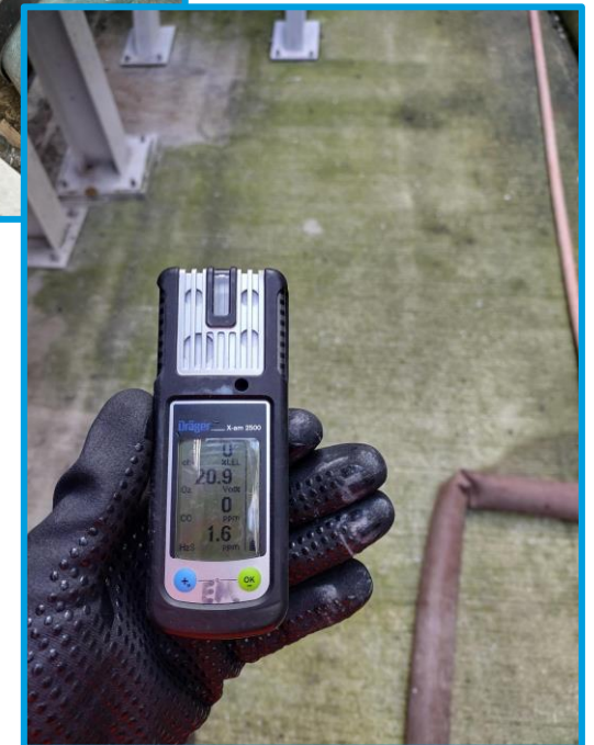
Personal Gas Detection Monitoring in area
