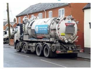
A temporary treatment unit used to treat excess groundwater and sewage then return this to a river
