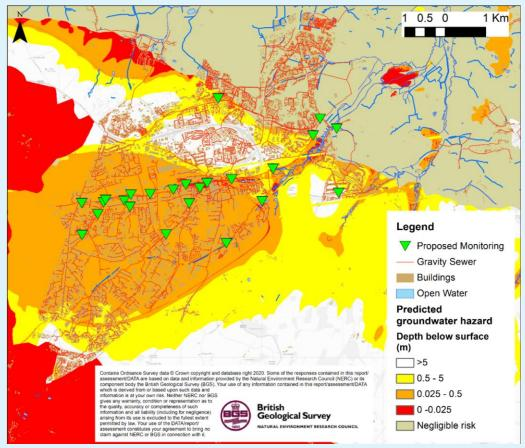
Figure 2.0 – Basingstoke monitoring plan area and infiltration zones
