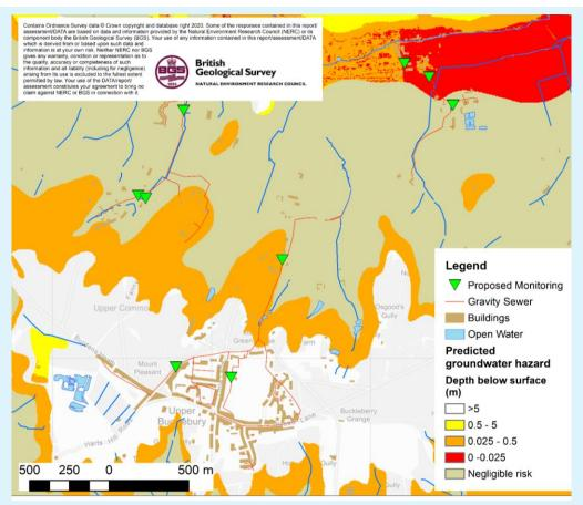
Figure 2.0 – Briff Lane (Bucklebury) monitoring plan area and infiltration zones
