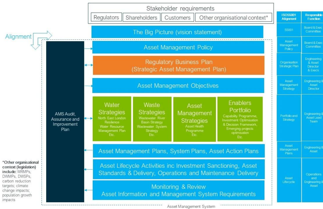
Figure 1 – Asset Management System Framework
