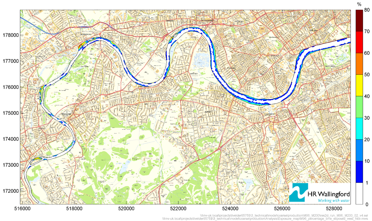
Figure A-33 Mogden scheme M96 baseline percentage of time intertidal exposure (14 – 29 November) during Richmond Pound November drawdown period
