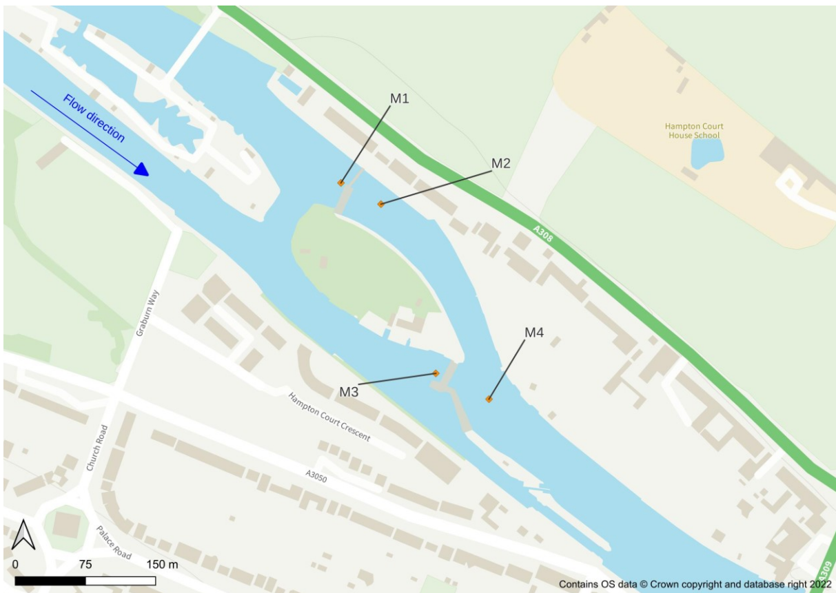
Figure A-30 Water level extraction points at Molesey Weir
