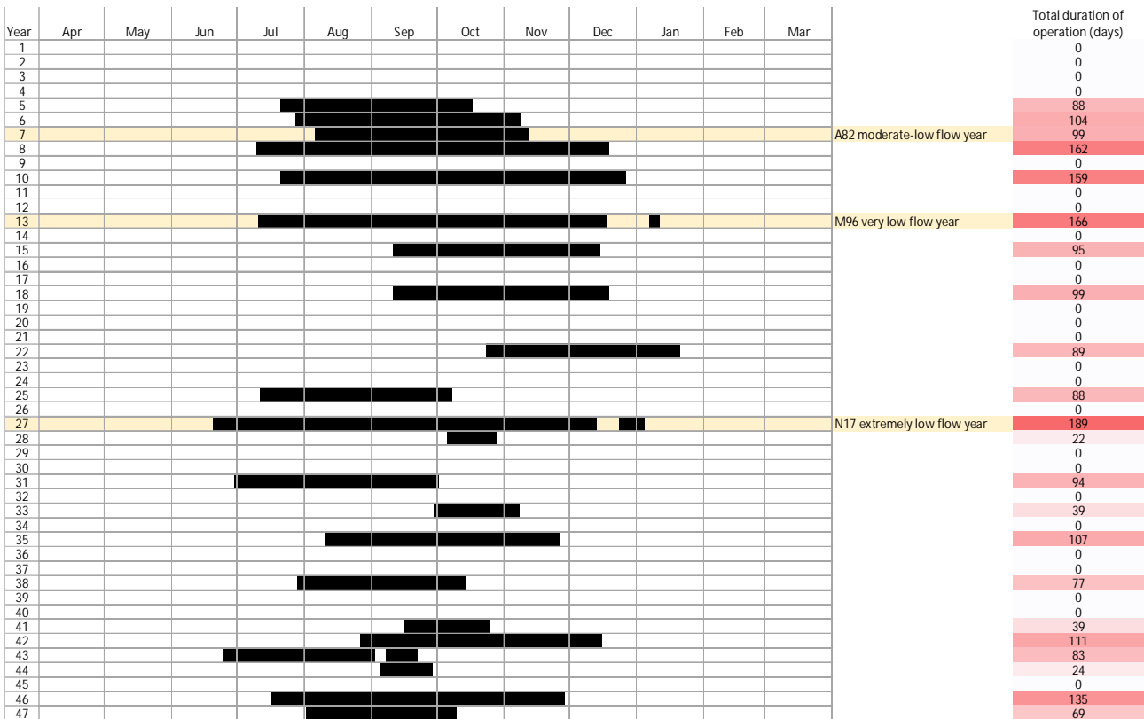
Figure 4-2: Based on Pywr Water Resources Modelling Using Strategic Schemes Trigger, expected duration of usage of a London water recycling scheme per water resources year
