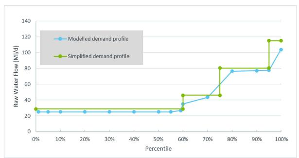
Figure 6-2: Operational utilisation profile for the 100Ml/d DO
