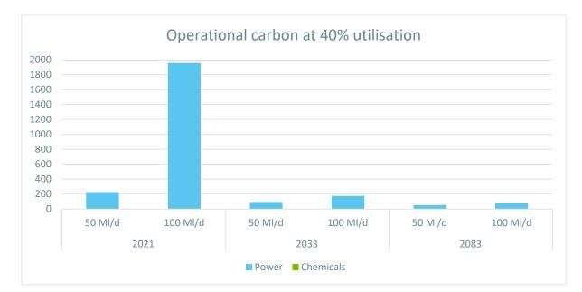
Figure 3-2: Operational carbon for 40% average utilisation profile at the ADO of 100MI/d and 50MI/d
