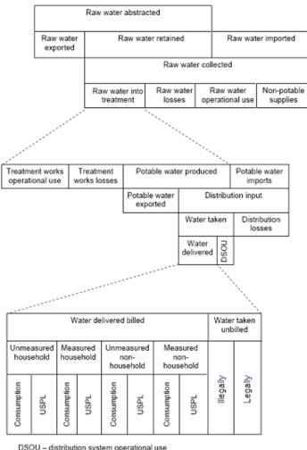
DSOU – distribution system operational use USPL – underground supply pipe losses
