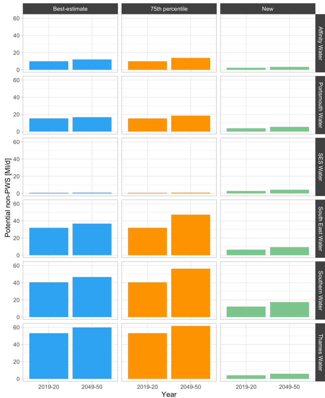
Figure 37 Non PWS in base year and 2050 by company split out by best and 75 th percentile estimate and new abstractions
