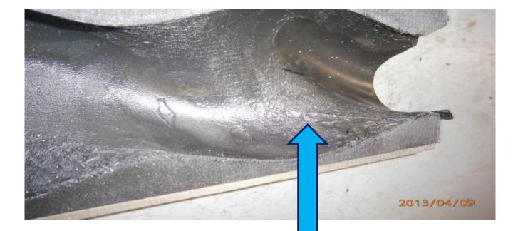
The inner surface of a run dry stator is hard and has a very rough texture. The pump dry running can cause the stator to burn creating a loss in performance.
