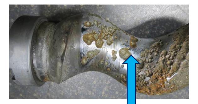
Chemical attack undermining the carbon steel base metal through the chrome plating.
