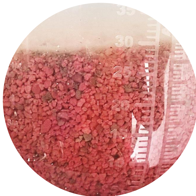
Anammox granules in use at pilot scale
