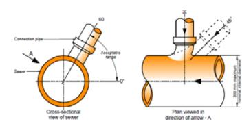
Make junction connections squarely and accurately by cutting the existing sewer with the appropriate machinery, and join the junction to the existing sewer using proprietary coupling/band seals.
