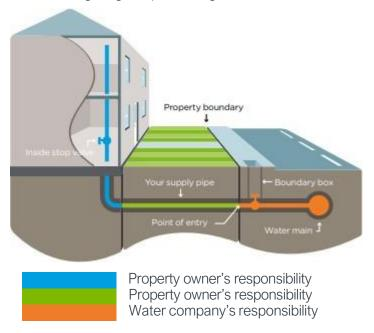
The supply pipe shall be the property owner's responsibility and shall conform to the Water Regulations and requirements of the Water Company.
