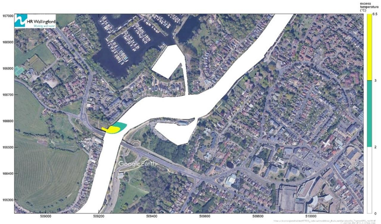
Figure 4-11 Temperature change in River Thames at outfall of 200 MI/d Mogden water recycling scheme at 780 MI/d river flow
