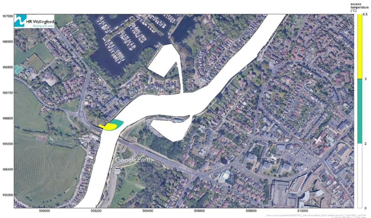
Figure 4-18 Temperature change in River Thames at outfall of 200 MI/d Mogden water recycling scheme at 950 MI/d river flow
