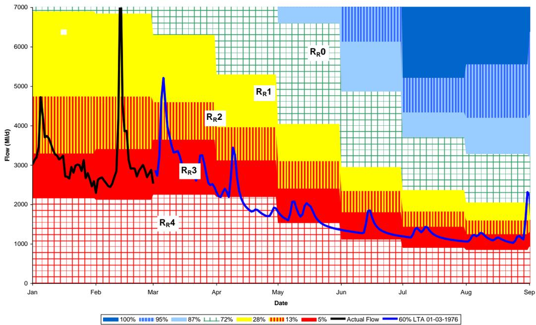
Figure 36 Flows over Teddington Weir, observed for January and February 1976 and predicted from March to August 1976 using 60% LTA. Bands show %ile splits based on 1900-2006 data.
