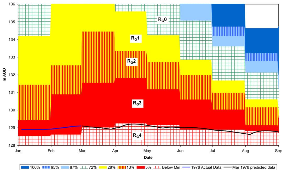
Figure 42 Groundwater Levels at Rockley showing actual data for January and February 1976 and predicted trend from March to August 1976. Bands showing % based on EA data.
