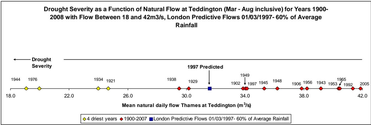
Figure 50 Potential Drought Severity from March 1997 Given Current Hydrological Indicators, Produced WARMS Model 6 Months Forecast at 60%LTA Rainfall
