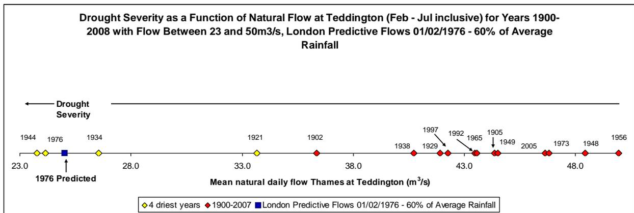
Figure 38 Potential Drought Severity from February 1976 Given Current Hydrological Indicators, Produced WARMS Model 6 Months Forecast at 60%LTA Rainfall
