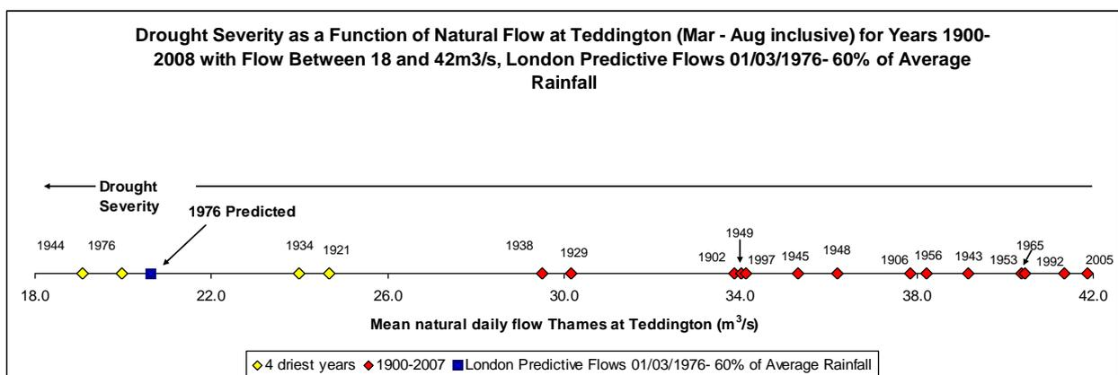
Figure 39 Potential Drought Severity from March 1976 Given Current Hydrological Indicators, Produced WARMS Model 6 Months Forecast at 60%LTA Rainfall
