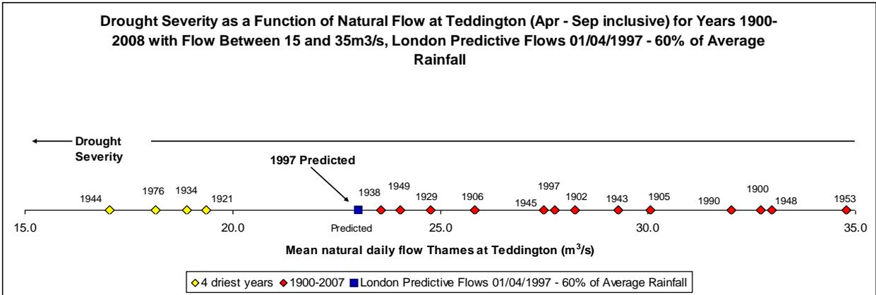
Figure 51 Potential Drought Severity from April 1997 Given Current Hydrological Indicators, Produced WARMS Model 6 Months Forecast at 60%LTA Rainfall
