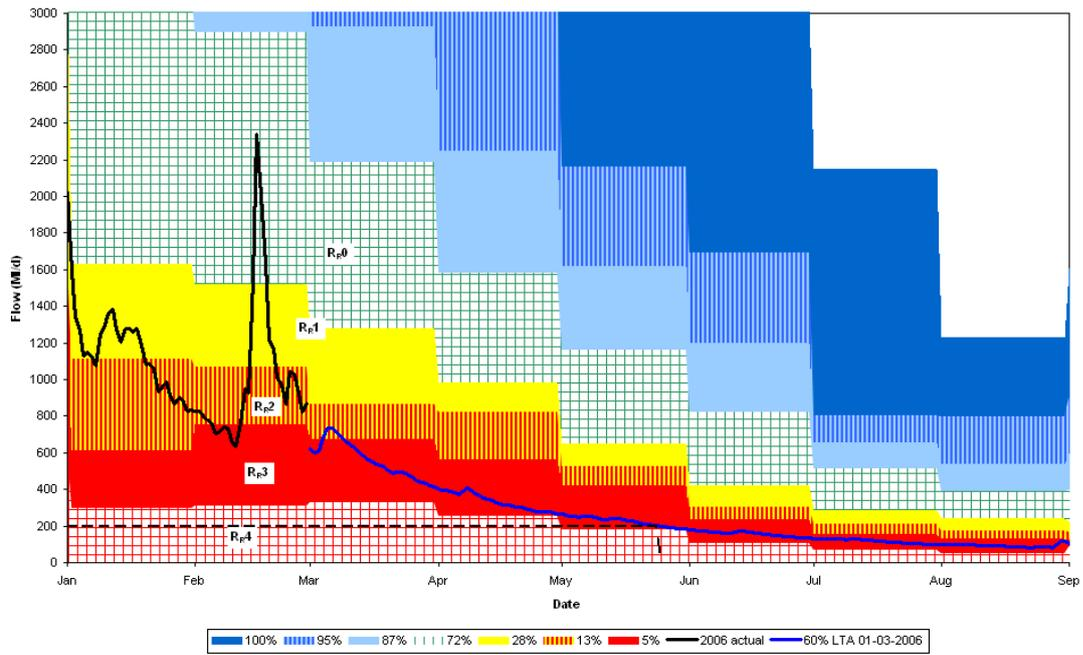
Figure 32 Prevailing flow January and February 2006 and Predicted River Flow at Farmoor between March and end of August, Bands Based on 1900-2006 Data for 60% LTA January to end of February
