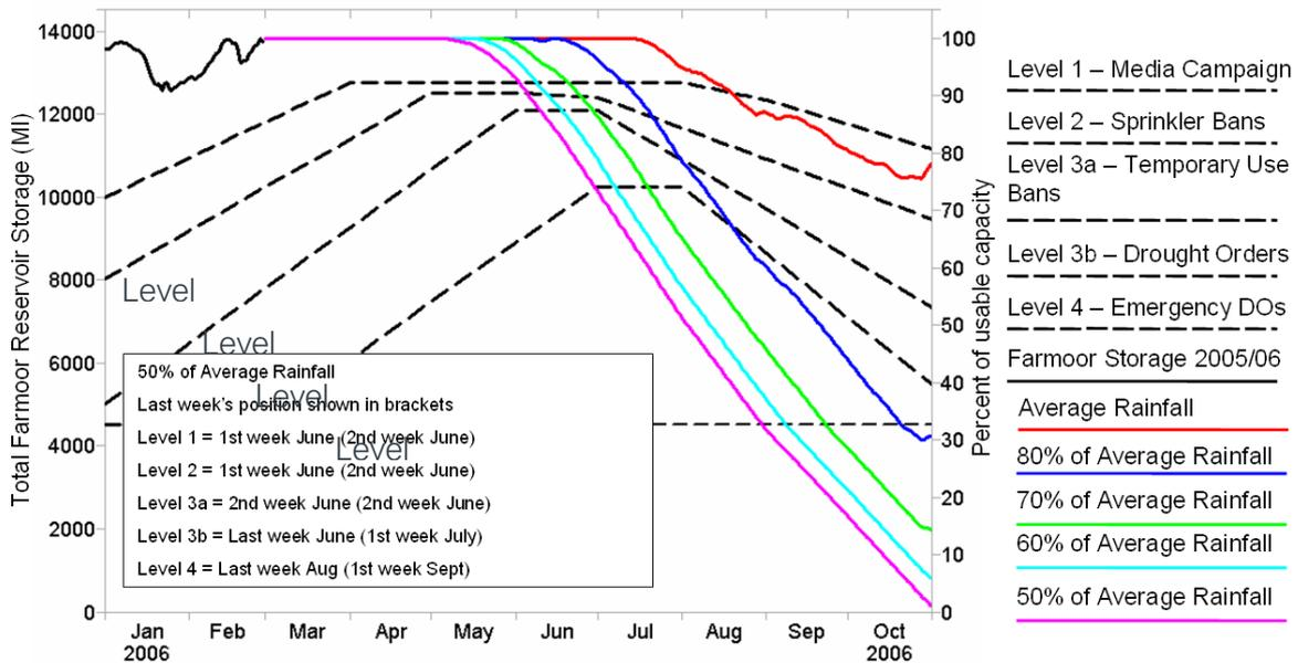
Figure 33 Predicted Reservoir Storage Showing prevailing storage from January to end of February 2006 and predicted storage using a 60% scenario from March to October 2006
