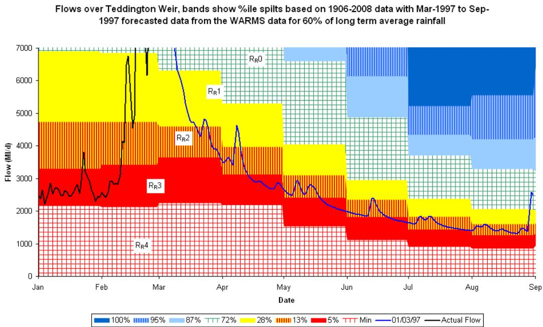
Figure 47 Flows over Teddington Weir, observed for January and February 1997 and predicted from March to August 1997 using 60% LTA. Bands show %ile splits based on 1906-2008 data.
