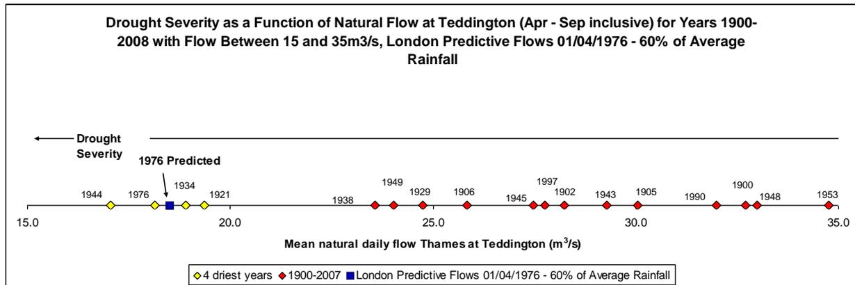
Figure 40 Potential Drought Severity from April 1976 Given Current Hydrological Indicators, Produced WARMS Model 6 Months Forecast at 60%LTA Rainfall
