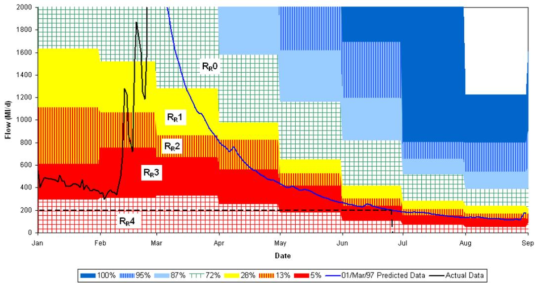
Figure 54 Flows at Farmoor, prevailing data from January to end of February 1997 and predicted flows from March to end of August 1997. Based on 60% LTA
