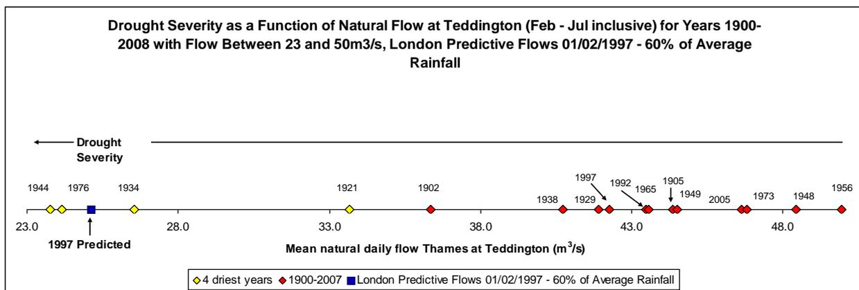
Figure 49 Potential Drought Severity from February 1997 Given Current Hydrological Indicators, Produced WARMS Model 6 Months Forecast at 60%LTA Rainfall
