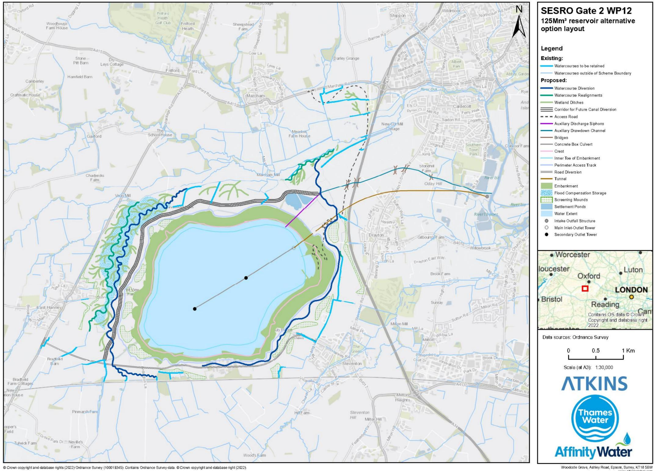
Figure 1.3 125 Mm<sup>3</sup> reservoir alternative option layout
