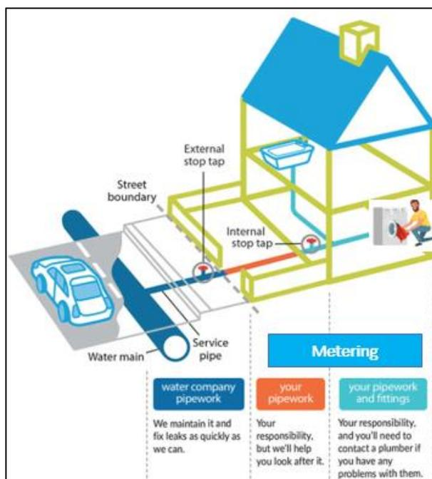
Figure 8-4: Water pipe ownership and metering<sup>15</sup>
