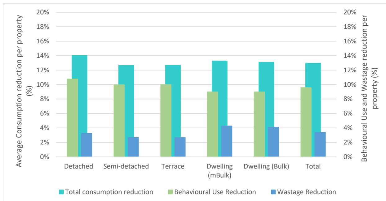
Figure 8-8: Smart metering consumption reduction (%) by property type
