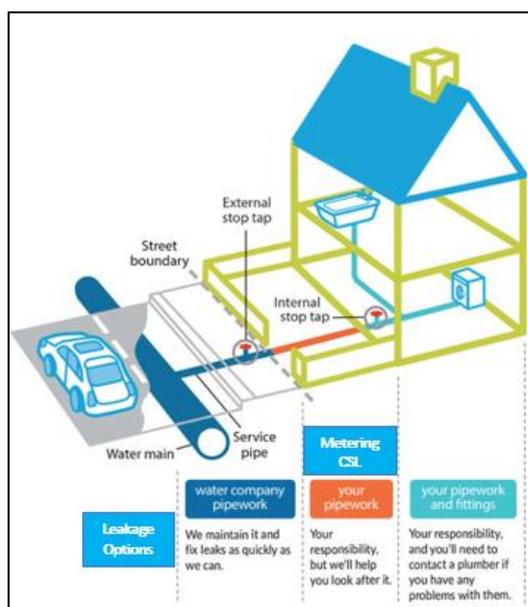
Figure 8-10: Water pipe ownership and leakage<sup>15</sup>
