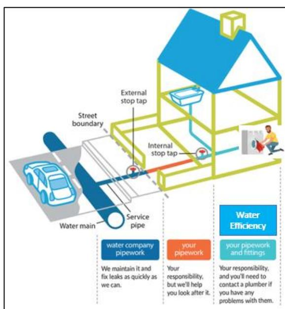
Figure 8-9: Water pipe ownership and water efficiency<sup>15</sup>
