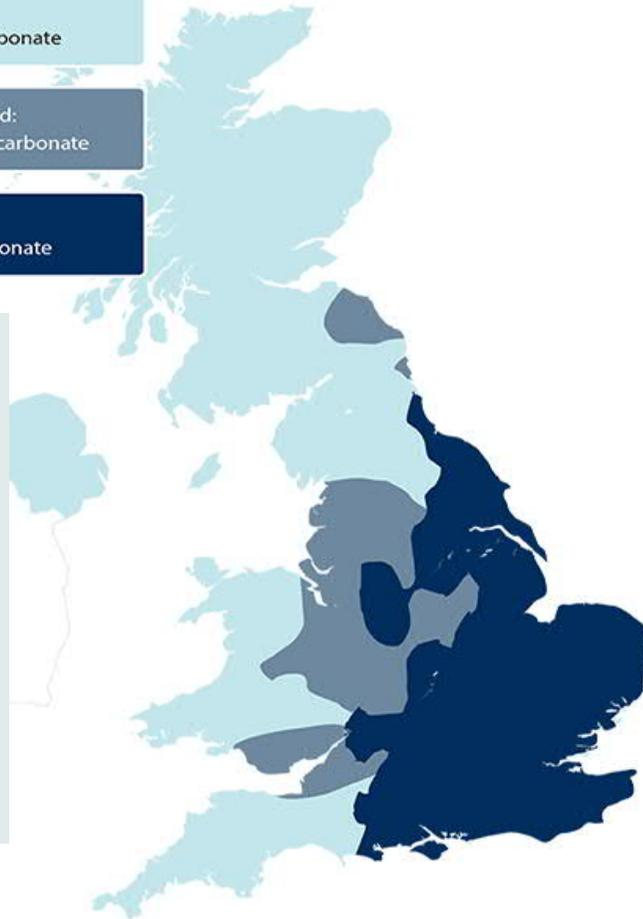
This map shows water hardness across the UK. When water falls as rain, it is 'soft' and free of minerals. It picks up naturally occurring minerals, such as calcium and magnesium, as it passes through rock, sand and soil, which causes the water to become 'hard'.
