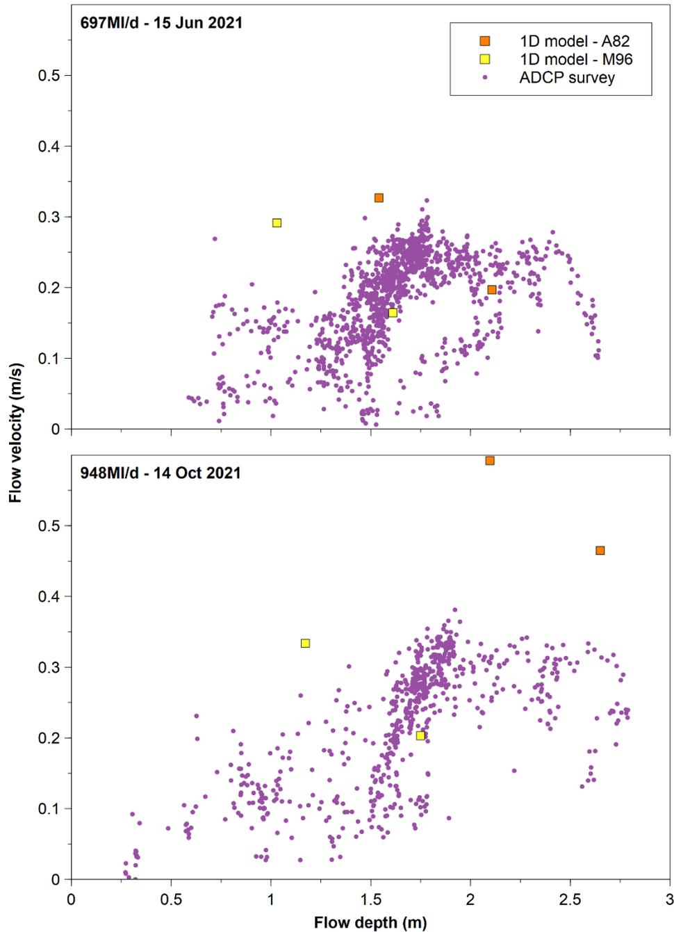
**Figure A 34** Montford ADCP and 1D model hydraulic data comparison
