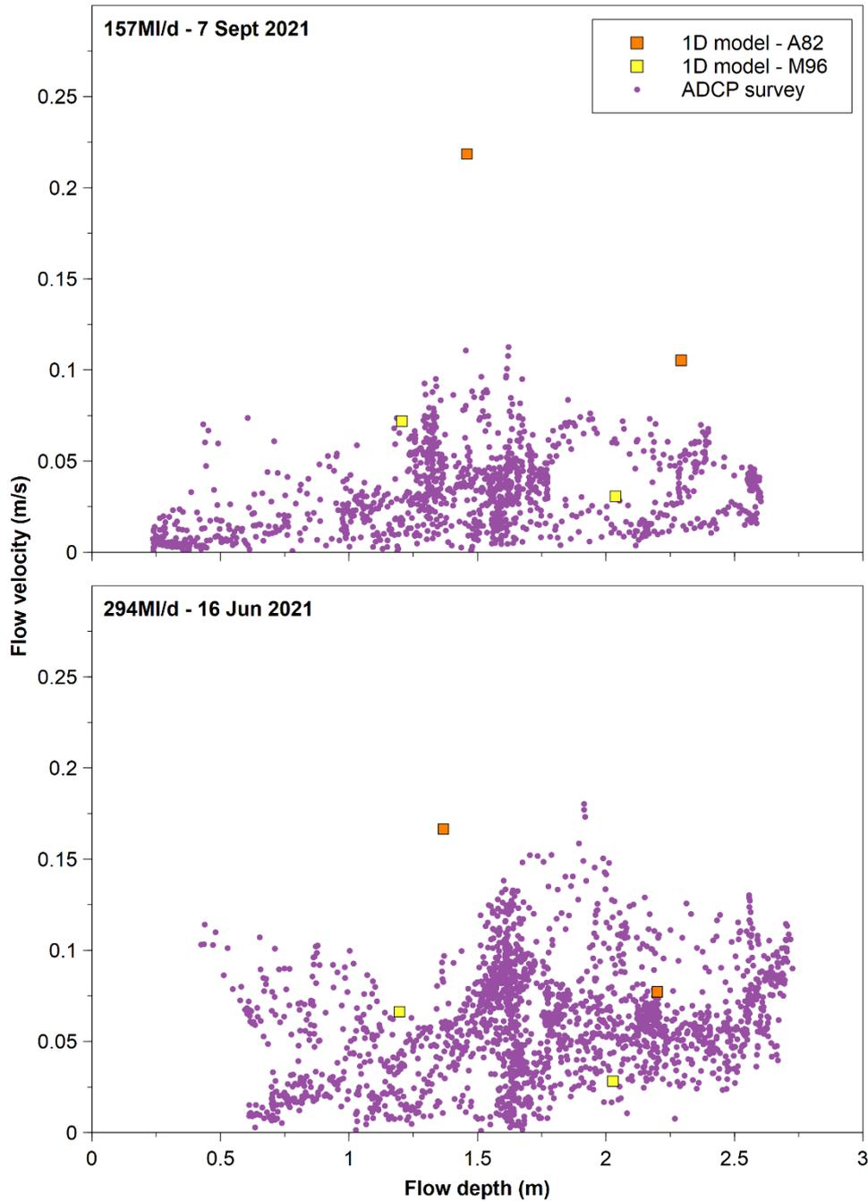
**Figure A 32** STT 5a ADCP and 1D model hydraulic data comparison
