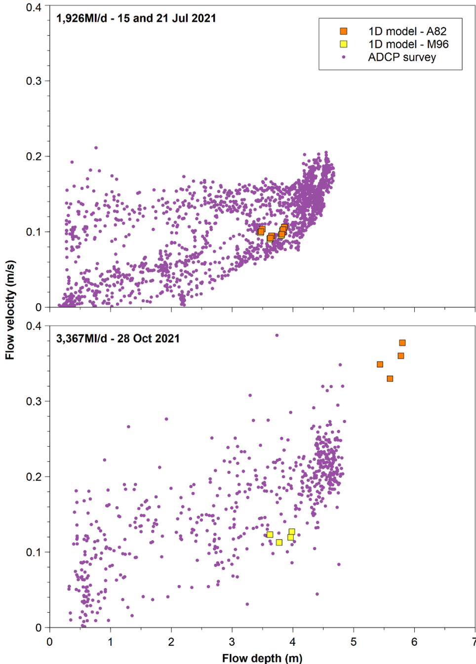
**Figure A 35** STT 10 ADCP and 1D model hydraulic data comparison
