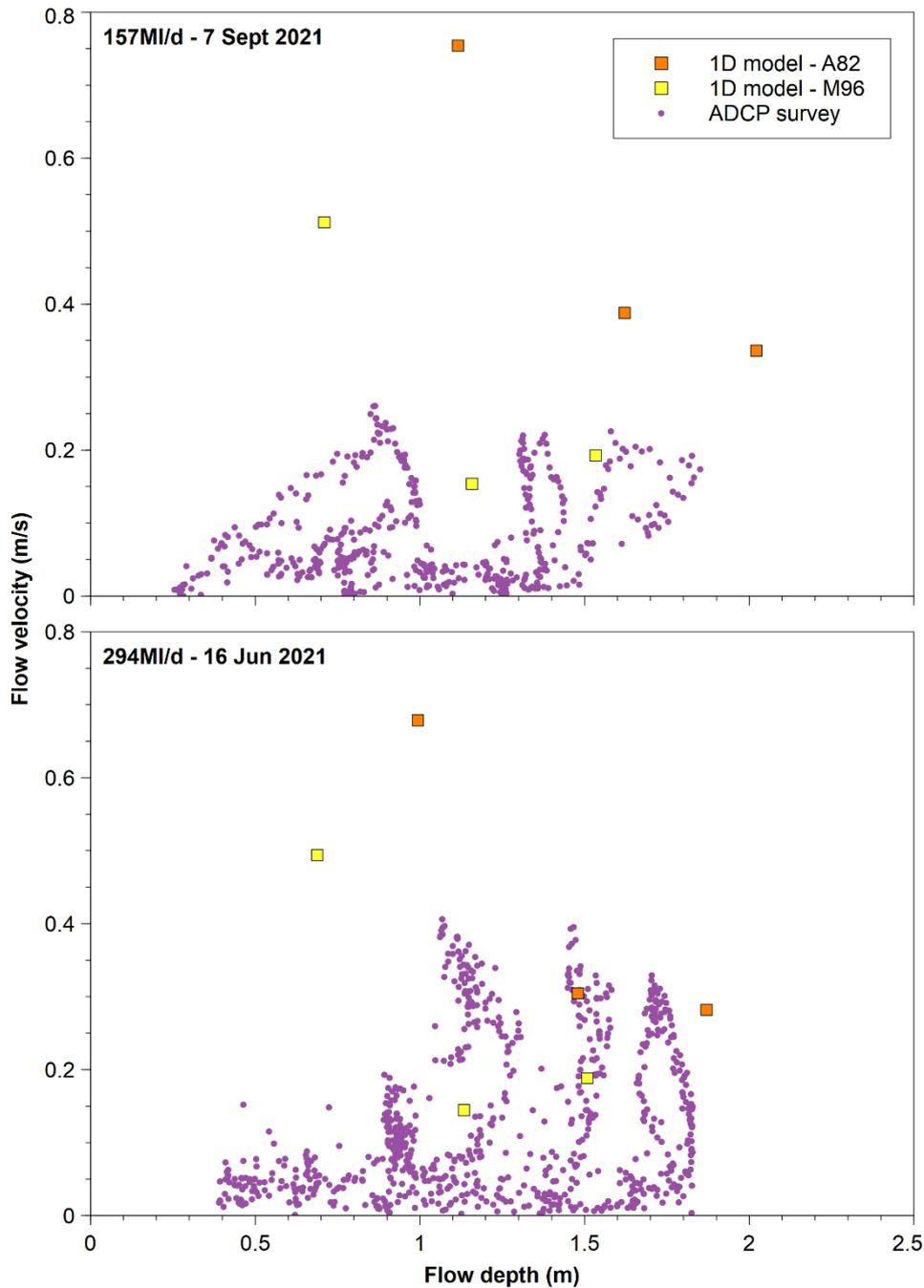
**Figure A 33** STT 5b ADCP and 1D model hydraulic data comparison
