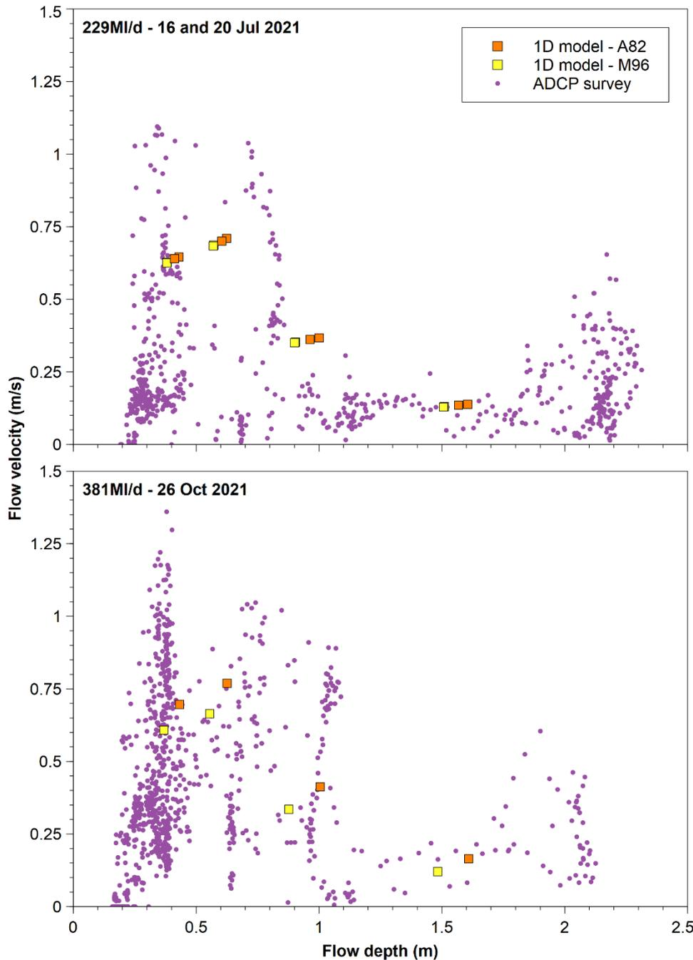
**Figure A 36** STT8 ADCP and 1D model hydraulic data comparison
